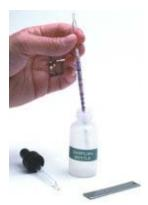
When specifications require safe and reliable testing for chloride contamination use CHLOR\*TEST "W". Each kit contains everything needed to perform five (5) individual tests.
